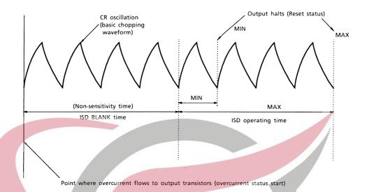
A non-sensitivity time is set for the overcurrent protector circuit to avoid misdetection of overcurrent due to spike current at irr or switching.
