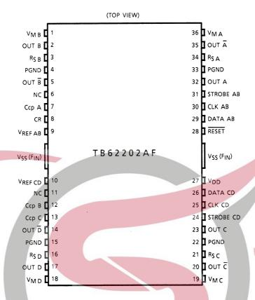
Note: [Important] If this IC is inserted reverse, voltages exceeding the voltages of standard may be applied to some pins, causing damage.
