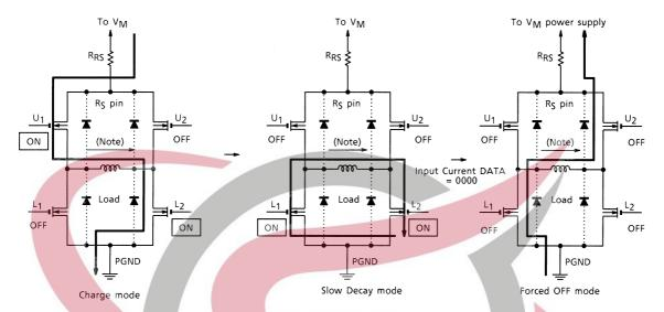
As shown in the figure at right, an output transistor has parasitic diodes.
